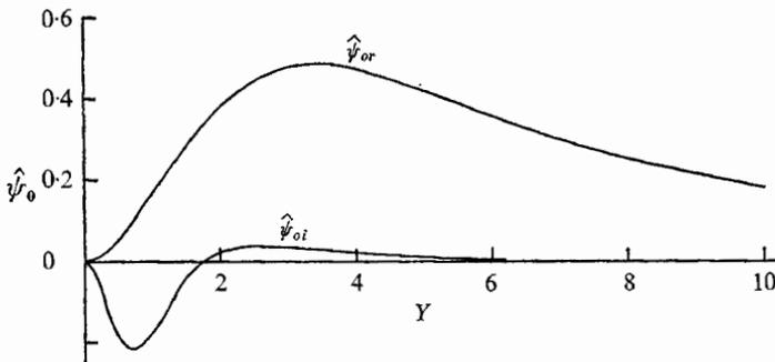
FIGURE 3. Eigenfunction  $\hat{\psi}_0$  for Blasius flow at  $\alpha = 0.172$ ,  $R_0 = 302.4$ .
