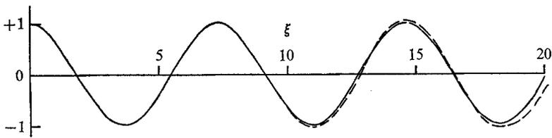
FIGURE 6. Streamwise growth of disturbance for Blasius flow at  $\alpha_0 = 0.072$ ,  $R_0 = 302.4$ :
