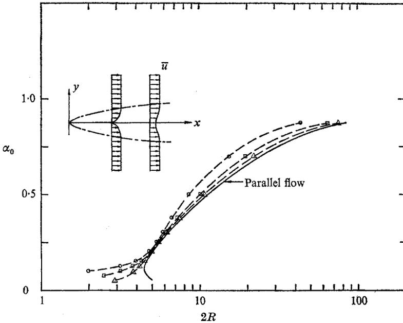
FIGURE 11. Neutral stability curves for the flat-plate wake. Non-parallel flow corrections:  $\circ$ ,  $0.664 \times (\pi x_0/l)^{-\frac{1}{2}} = 2$ ;  $\square$ , 1;  $\triangle$ , 0.5.
