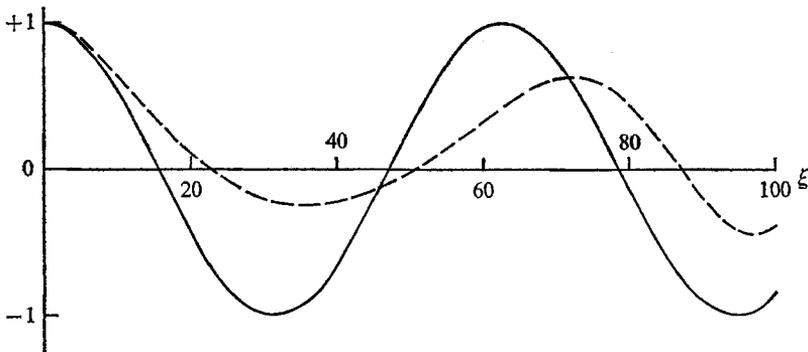
FIGURE 12. Streamwise disturbance behaviour for the flat-plate wake at  $\alpha_0 = 0.1, R_0 = 2.26$ . —,  $\text{Re}(\exp\{i\alpha_0\xi\})$ ; ----,  $\text{Re}(\exp\{i\alpha\xi\})$ .
