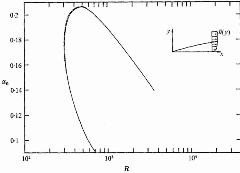
FIGURE 1. Neutral stability curves for Blasius flow: —, parallel flow; - - -, non-parallel flow.
