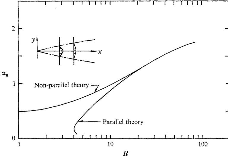
FIGURE 7. Neutral stability curves for the two-dimensional laminar jet.
