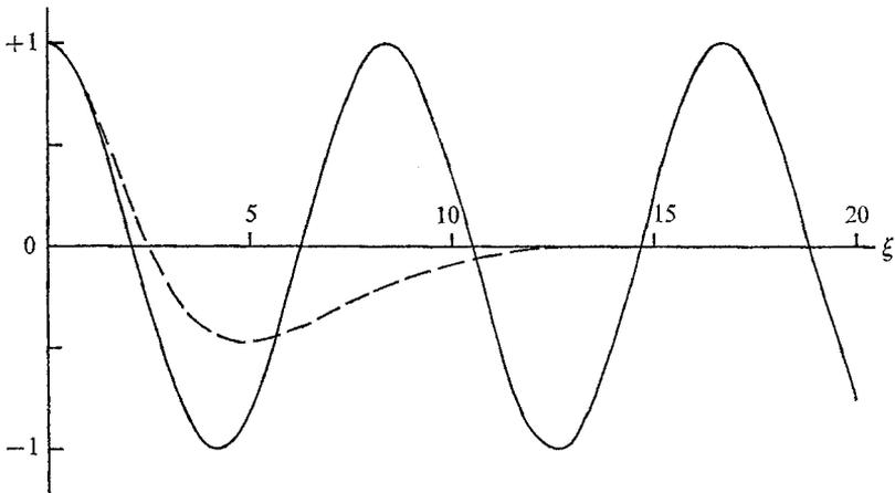
FIGURE 8. Streamwise disturbance behaviour for the two-dimensional laminar jet at  $\alpha_0 = 0.75$ ,  $R_0 = 8.21$ : —,  $\text{Re}(\exp\{i\alpha_0\xi\})$ ; - - - ,  $\text{Re}(\exp\{i\xi\})$ .
